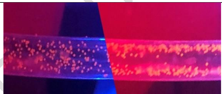
Microplastics naturally scatter in flowing water (left), but after turning on sound waves, the particles concentrate along the tube’s sides (right), making them easier to remove.
